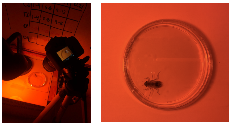
Figure 1: Viewing chamber for recording ventilation rates of dragonfly nymphs. Left: Camera set-up. Right: Viewing chamber orientation under the camera.
